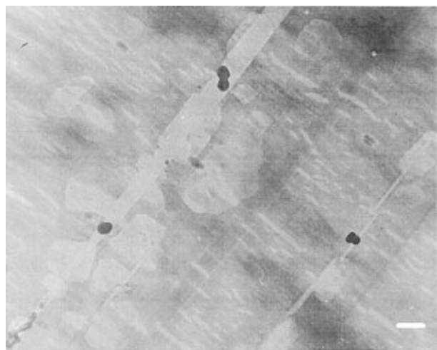
Figure 3. Bright field electron micrograph of a thin film of POBA epitaxially oriented on PTFE ( T_{\text{polymerization}} = 210\text{ }^{\circ}\text{C} ; scale bar = 50 nm).
